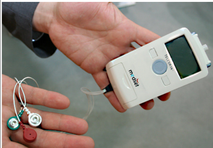
A direct-methanol micro fuel cell powers an iPhone-sized mobile electrocardiogram recorder developed by the German Medset company. It's scheduled to be ready for market by the end of the year. (Photo by Sven Geitmann)
