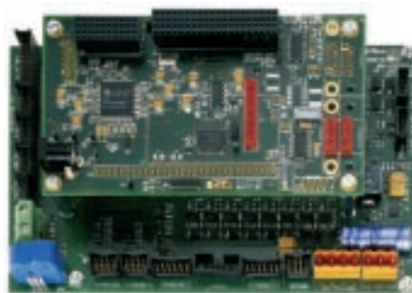
Control system based on a microprocessor.
