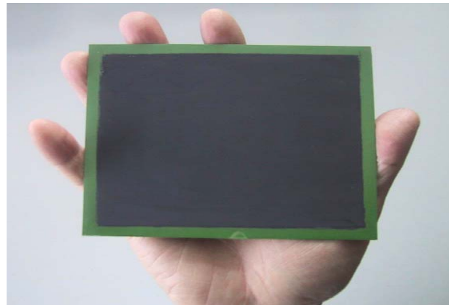
Planar Cells Effective area: 100 cm 2 Cell power: > 50 W at 0.7V
