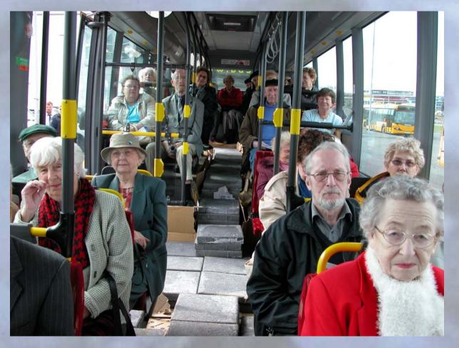
To reach a full load of the vehicle we filled the floor with concrete tiles.
