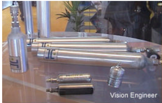
Hydrogen storage containers (with metal alloys inside)
