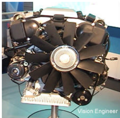
The BMW Hydrogen 7 Series IC Engine (135KW power output)
