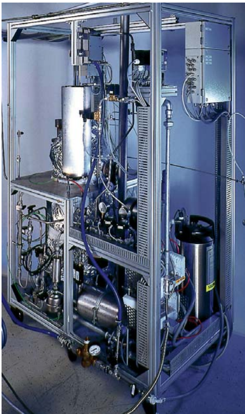
Natural gas reformer for a 2 kW el fuel-cell CHP plant.
