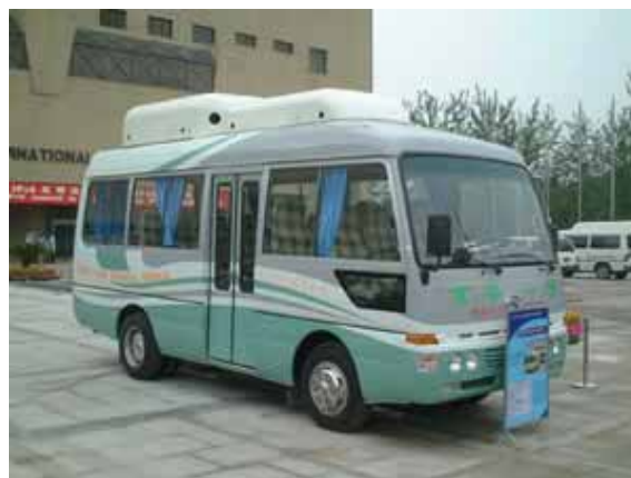
Fig.12: PEM fuel cell bus. Source: Tsinghua University
